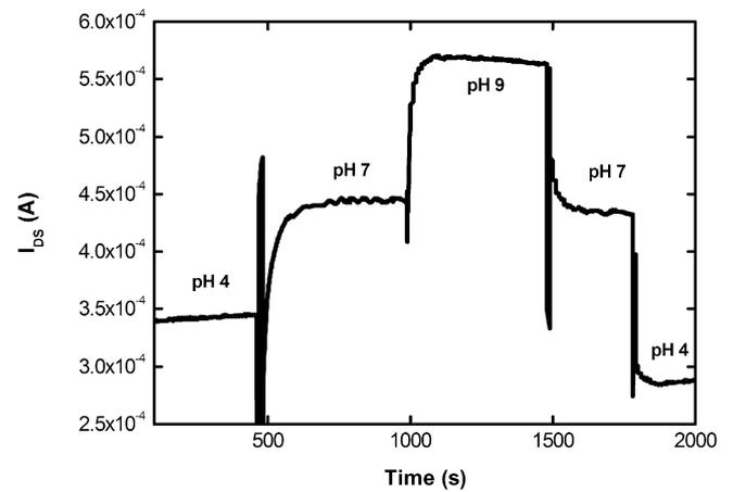
Fig. 4. pH sensitivity of the floating-gate FET with  $V_{D5} = V_{G5} = -1 \text{ V}$  in buffers with pH 4, 7, 9.
