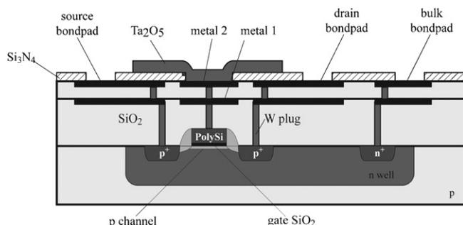
Fig. 1. Cross-section of the p-channel floating-gate FET.
