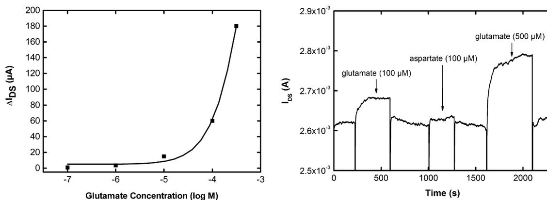
**Fig. 5.** (A) The change of the drain current of the transistor in function of the logarithmic glutamate concentration in PBS, pH 7. (B) ENFET response upon injection of glutamate (100  $\mu\text{M}$ ), aspartate (100  $\mu\text{M}$ ) and glutamate (500  $\mu\text{M}$ ). The measurement was started in PBS buffer (150 mM, pH 7), and changed to glutamate in PBS, aspartate in PBS and back to glutamate. The device was measured in constant voltage mode and biased with  $V_{DS} = V_{GS} = -1$  V.
