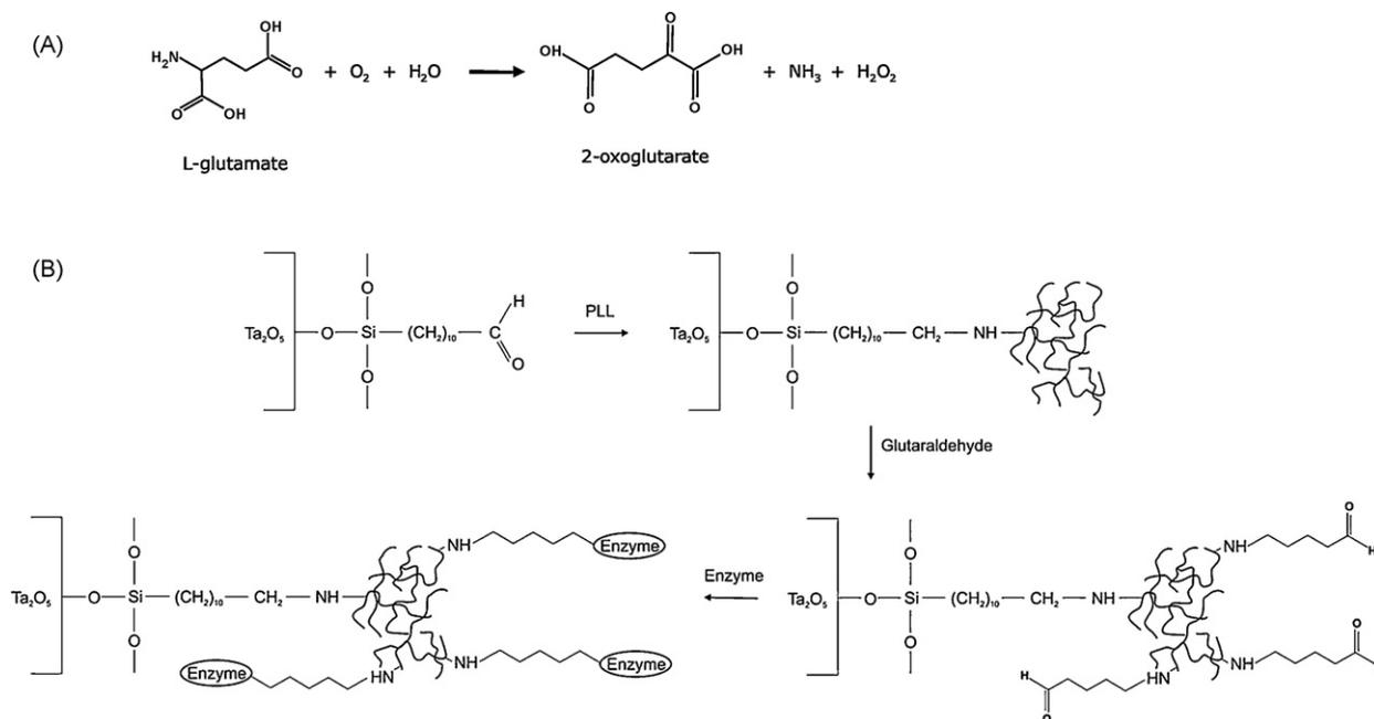
**Scheme 1.** (A) Reaction scheme of the conversion of glutamate by glutamate oxidase (GLOD). (B) Reaction scheme of the immobilization of GLOD on the chips using silane SAMs, PLL and glutaraldehyde.
