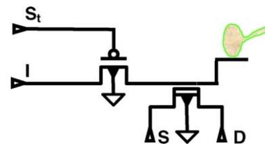
Fig. 2. Combined sensing and stimulating transistor: (S) source; (D) drain; (I) electrode for neuron stimulating pulses; ( $S_t$ ) the switching control.
