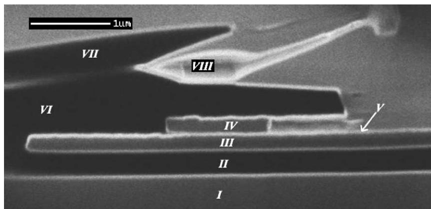
Fig. 3. Inclined cross-section SEM picture of the edge of the FG structure after focused ion beam etch. The various layers are: (I) silicon substrate; (II) 0.5 µm field oxide; (III) bottom polycrystalline silicon layer; (IV) remained upper PS layer; (V) 420 Å of thermal oxide layer between the two PS layers; (VI) PSG; (VII) oxynitride passivation layer; (VIII) artifact of the FIB platinum deposition. The bottom PS layer acts as the FG.
