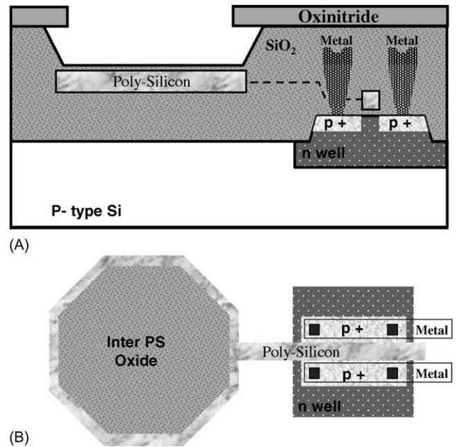
Fig. 1. (A) Cross-section of the FG transistor. The substrate is p-type Si. The p-channel transistor is located inside the n-well. The p+ indicates the source and drain regions. The gate oxide is 115  $\text{\AA}$  thick. The poly-silicon electrode is covered by thermal oxide of 420  $\text{\AA}$ . (B) Top view of the FG transistor.
