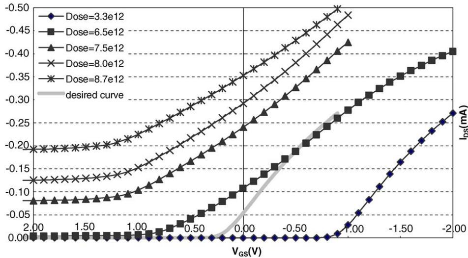
Fig. 4.  $I_{DS}$  vs.  $V_{GS}$  at  $V_{DS} = 0.1$  V and  $V_{BS} = 0$  V for different boron ion implantation doses. The desired device curve is also shown.
